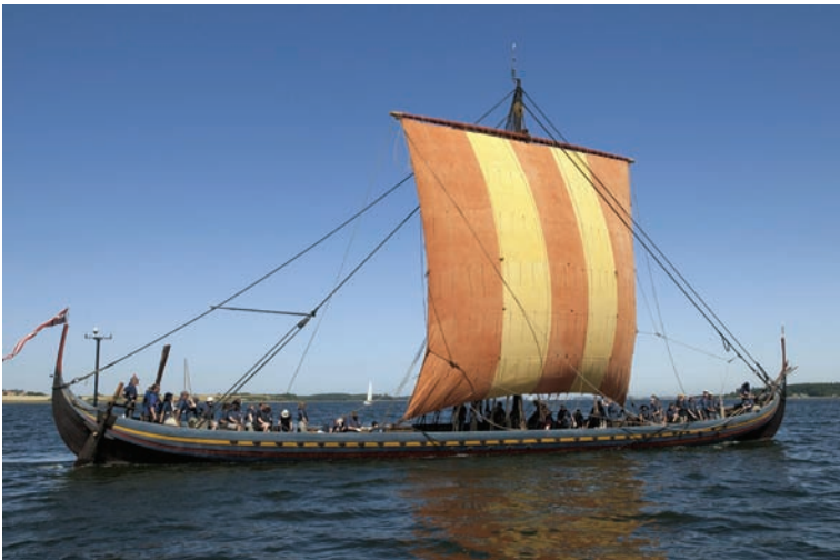
PLATE 6. The Viking Ship Museum in Roskilde, Denmark, used medieval shipbuilding techniques in creating a reconstruction of one of the grandest Viking longships ever found by archeologists. “The Sea Stallion of Glendalough” has proven eminently seaworthy and has sailed from Denmark to Dublin and back; volunteers have the opportunity to man the oars every summer. Photo: Vikingskibsmuseet, Roskilde. Reproduced with permission.
